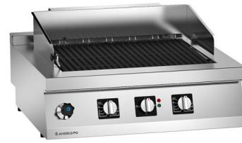
Grill range made of AISI 304 stainless steel, 20/10 mm thickness top. Cooking griddle made of enamelled cast iron with special nanotechnology surface treatment for a better fats sliding, delivered with stainless steel splash guards and cleaning brush. Heating by two independent tilting electric heating groups. Lower well, water filling through tap with adjustment knob, capacity 13 lt (overflow).
